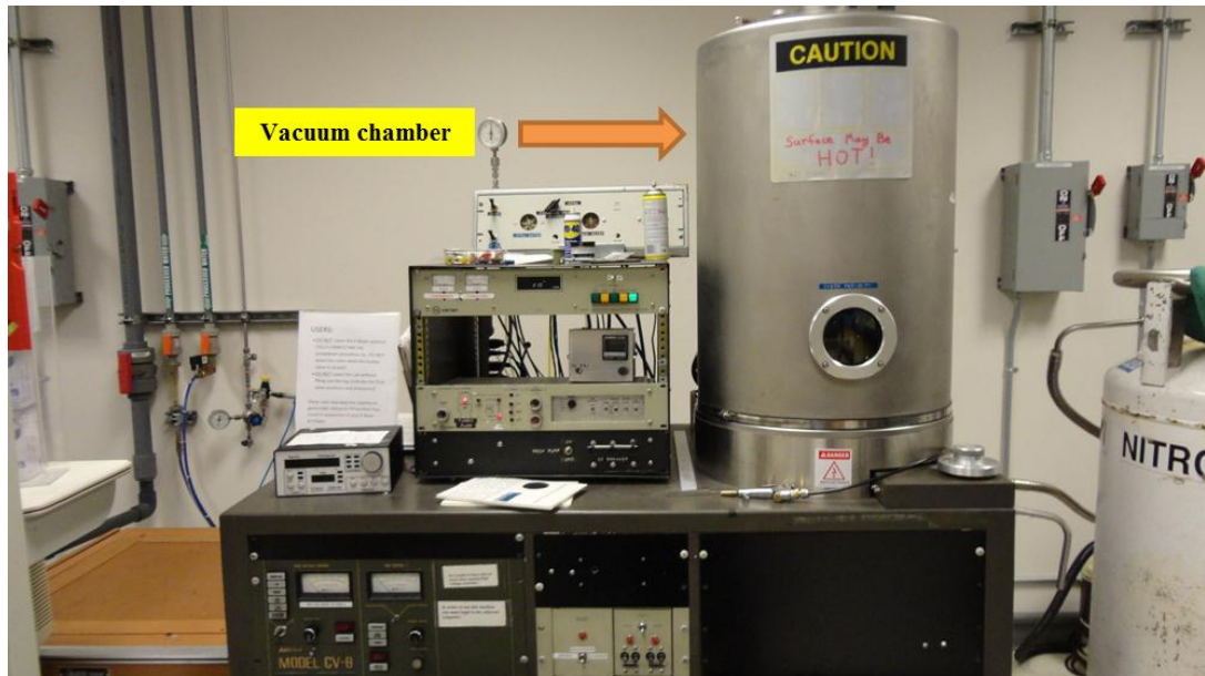
Fig. B1 E-Beam Evaporator at NREC
